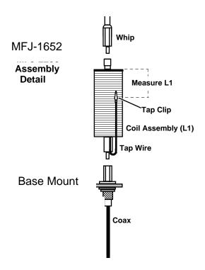
[ ] Install coil assembly with tap-wire end toward the Base Mount.
